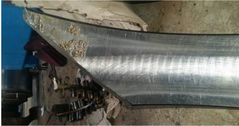
Image 4. Outer race damage.
