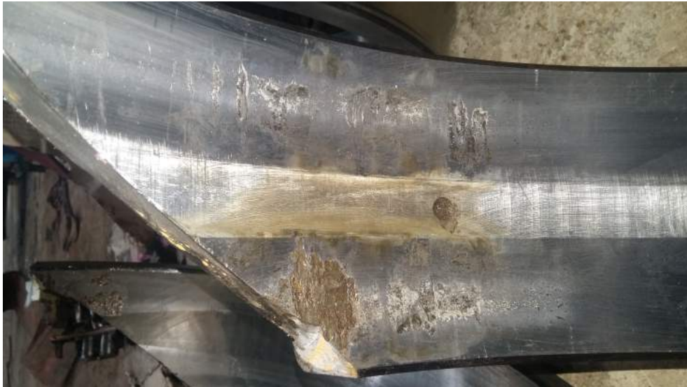
Image 2. Damage to the bearing outer race.
