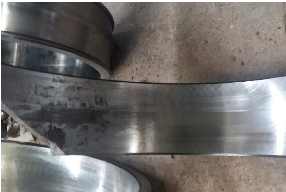
Image 3. Outer race bearing damage.
