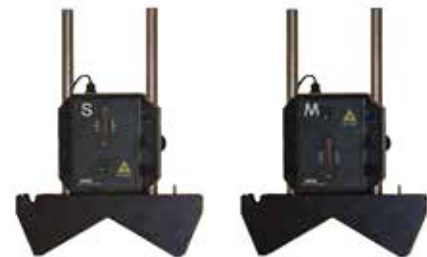
The alignment sensors are identical with exception of the position of laser diode and the knob for adjustment of the laser on the 'M' sensor. Sensor size: 86x81,5x36 mm, weight: 230 g
