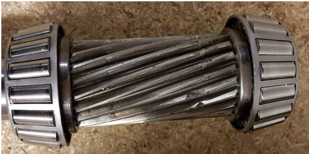
Img. 5 Damaged input shaft gear.
