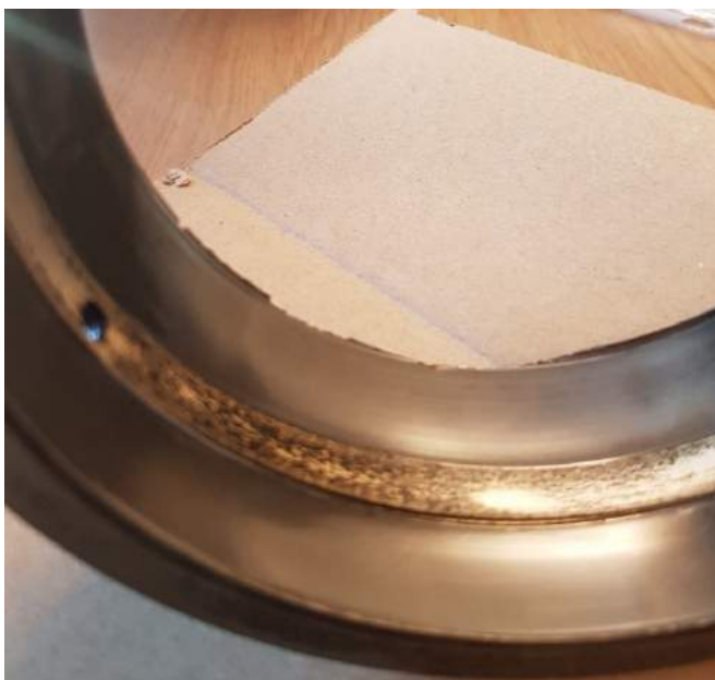
Img. 2 Damaged bearing from the 1 st intermediate shaft.
