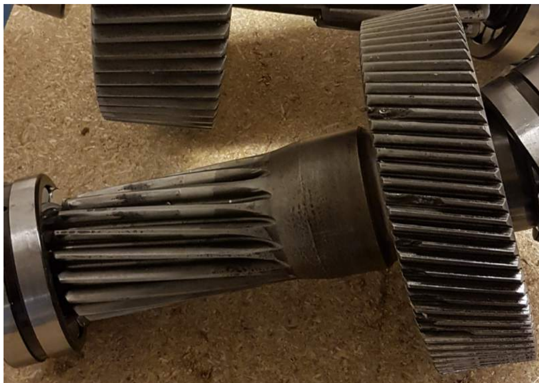
Img 4. Damaged 1 st intermediate shaft.
