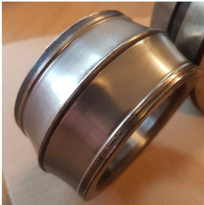
Img. 1 Damaged bearing from the 1 st intermediate shaft.
