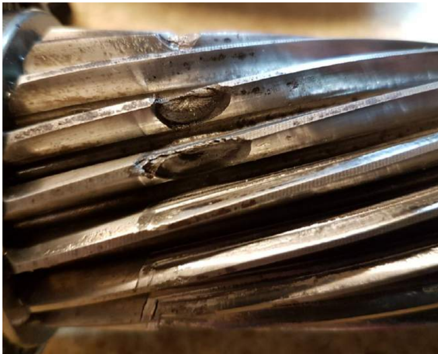
Img. 6 Damaged input shaft gear.
